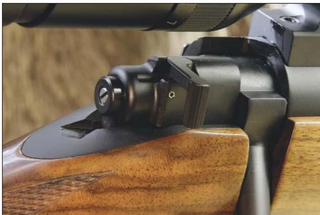
Left, the original Kimber tang has been slightly reshaped, as has the bolt root. Note the three-position wing safety. Above, the original Kimber floorplate was nicely fitted.
