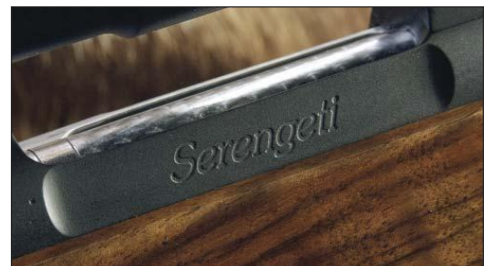
Left, the bolt root and trigger have been modified from the Kimber original. Talley one-piece aluminum mounts are in keeping with the light weight and smooth lines. Below, a flat milled on the side of the action reduces weight and provides a canvas for the maker's name, Serengeti.
