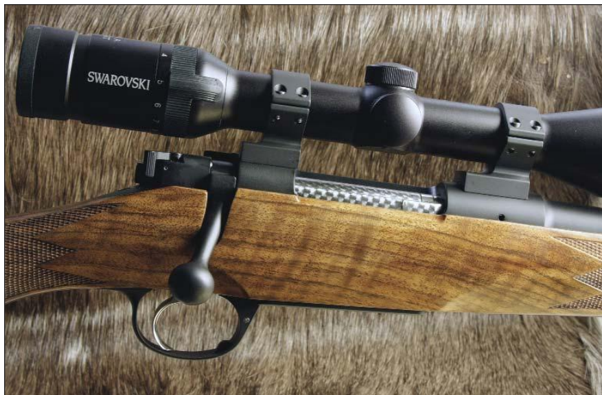
Left, the bolt root and trigger have been modified from the Kimber original. Talley one-piece aluminum mounts are in keeping with the light weight and smooth lines. Below, a flat milled on the side of the action reduces weight and provides a canvas for the maker's name, Serengeti.
