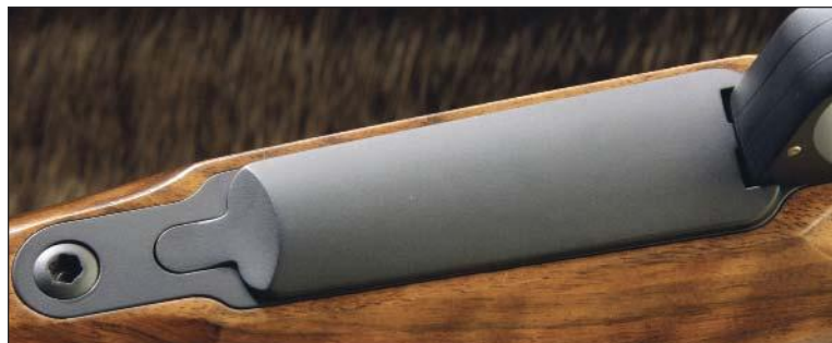
Left, the original Kimber tang has been slightly reshaped, as has the bolt root. Note the three-position wing safety. Above, the original Kimber floorplate was nicely fitted.
